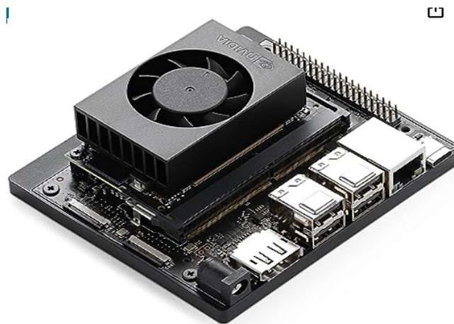
*Figura 5. NVIDIA Jetson Orin Nano Developer Kit*
