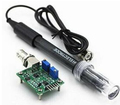
Figura 10. Sensor de pH GAOHOU PH0-14
