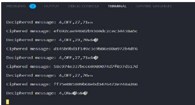
Fig. 14: ESP-NOW mesh data encrypted with AES.
