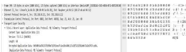
Fig. 15: MQTT data encrypted with TLS.
