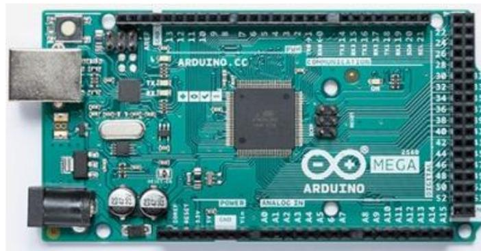
Figura 9: Arduino Mega 2560 [36]
