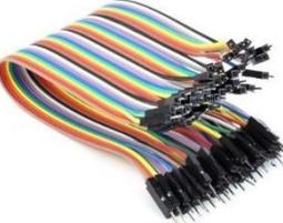
A rainbow-colored ribbon cable with two sets of female headers on both ends, used for connecting components to a protoboard. |
