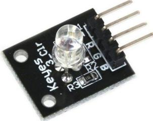
A small black PCB module with a clear LED lens in the center and four pins extending from the bottom. The text 'Keyes 12-3-Cl' and 'RGB' is visible on the board. |
