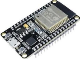
A black ESP32 development board with a gold-colored ESP32 chip, various components, and a USB-C port.                         |
